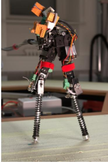
Figure 3: Bio-inspired dynamical bipedal walker using Bayesian Optimization
